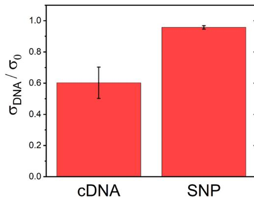
**Figure 7.** Biosensor Selectivity. Conductivity change in Au NP-decorated ZnO NW biosensors upon introduction of a 10 nM solution of a fully complementary DNA strand (cDNA) or a strand containing a single nucleotide polymorphism (SNP). Fully complementary strands induce a larger decrease in the ZnO NW conductivity. Error bars show the standard deviations taken from at least five samples.
