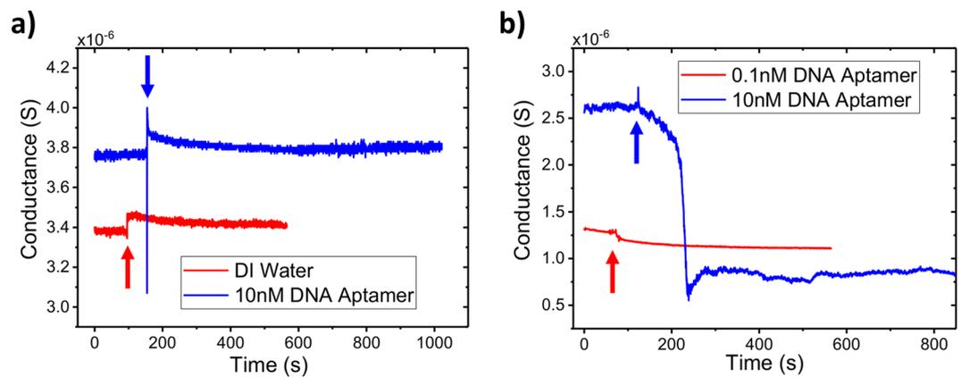
**Figure 4.** Biosensor response to thiolated DNA aptamer Conductance vs. time plots of bare (a) and Au NP decorated (b) single ZnO NW devices upon introduction (arrows) of 10  $\mu$ L of the indicated solution. The negatively charged thiolated DNA aptamer binds to the Au NPs on the NW surface, inducing positive charges and decreasing the ZnO NW conductivity; in contrast, DNA is unable to bind to the unmodified NW surface and solution introduction has no effect on conductivity.
