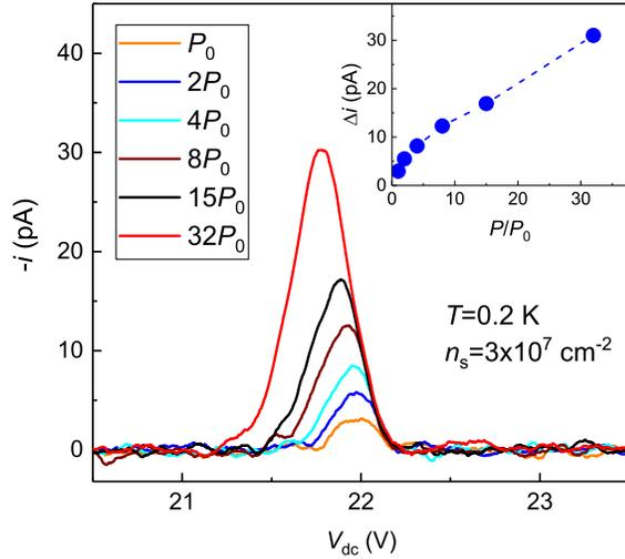
FIG. 3. The current signal measured at the top capacitor plate for SE irradiated with pulse-modulated MW at frequency  $\omega_0/2\pi = 140$  GHz for different MW power. Inset: The current signal at the resonance vs the normalized MW power.
