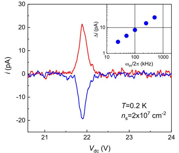
FIG. 2. The current signal measured at the bottom (red line) and top (blue line) capacitor plate for SE irradiated with pulse-modulated MW at frequency  $\omega_0 / 2\pi = 140$  GHz. (Inset) The current signal at the resonance measured for different values of the pulse-modulation frequency  $\omega_m$ .
