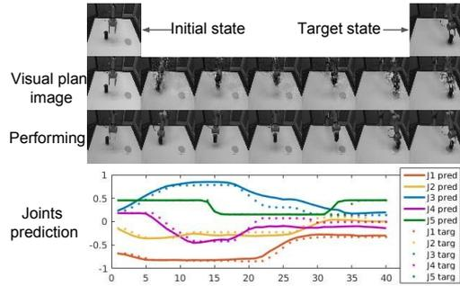
Figure 3: Example of plan generation. The top row shows images of the initial and target visual states, the second row shows the generated image sequence (sampled), and the third row shows the image sequence captured when the robot followed the plan, for comparison. The bottom row shows generated joint angles (solid lines) and ground truth joint angles from the experimenter (dotted lines)
