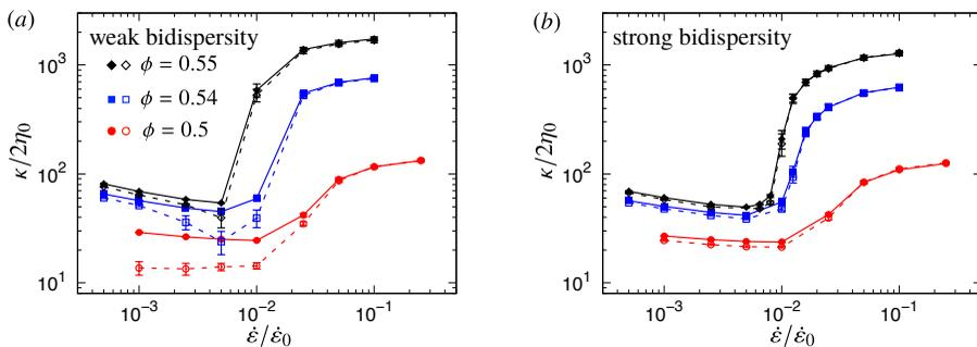
FIGURE 3. Mixing particles of different sizes hinders the shear-induced ordering. Differences in  $\kappa$  between extensional flow (filled symbols with solid lines) and simple shear (open symbols with dashed lines) are still present in the weakly bidisperse suspensions,  $a_2/a_1 = 1.2$  (a), but no longer significant in the strongly bidisperse suspensions,  $a_2/a_1 = 1.4$  (b).
