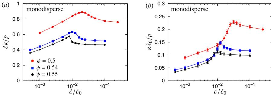
FIGURE 4. (a) The ratio between  $\dot{\epsilon}\kappa$  and  $p$  for monodisperse suspensions in extensional flows remains of the order of unity even when the viscosity increases significantly. (b) The positive values of the ratio  $\dot{\epsilon}\lambda_0/p$  for monodisperse suspensions in extensional flows indicate some anisotropy in the pressure response, namely the in-plane pressure is higher than the out-of-plane pressure.
