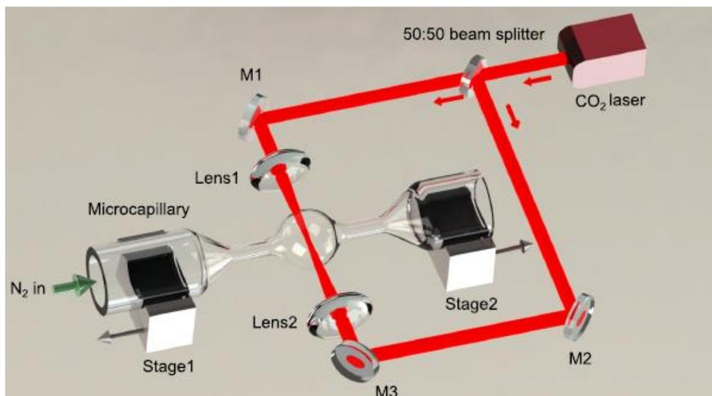
Fig. 1. Microbubble fabrication setup. A CO<sub>2</sub> beam is focused using two lenses (Lens1 and Lens2) onto a tapered silica glass capillary while internally pressurizing it using nitrogen gas. M1, M2, M3: mirrors.
