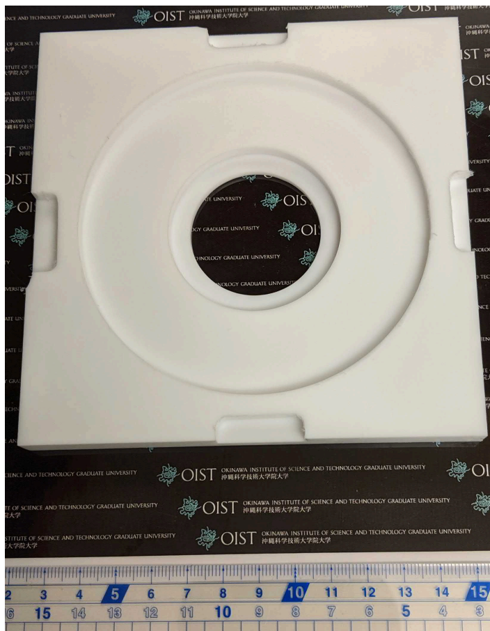
Figure D.2: The CNC milled PTFE casting station for PDMS soft lithography supporting 2-inch and 4-inch wafer.
