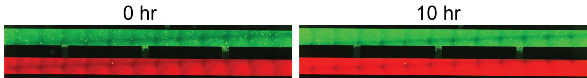
Figure 2.21: Stable chemical transport in double-layer PMMA/PDMS chip before and after 10 hours. Fluorescein-dextran was perfused in the top channel (Green) and tetramethylrhodamine-dextran was perfused in the bottom channel (Red).
