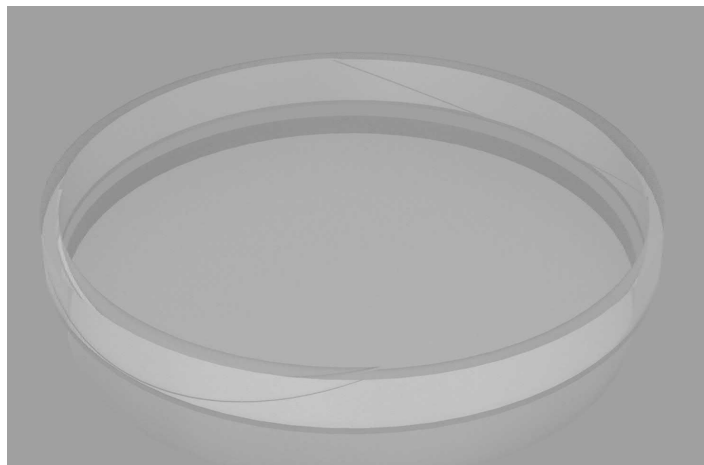
Figure B.16: Two-piece assembly approach. An outer ring with paraboloid structures and an inner cylinder that can be precisely mate with the outer ring.
