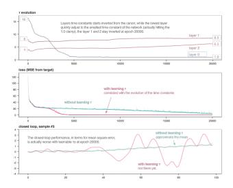
The loss of the network benefits from the adaptation of the  $\tau$  values. However, its closed-loop error actually is worse: the network with fixed  $\tau$  is mostly approximating the slow mean of the samples, while the network with learnable  $\tau$  is starting to learn to reproduce faster features of the patterns, but is not yet good at it.
