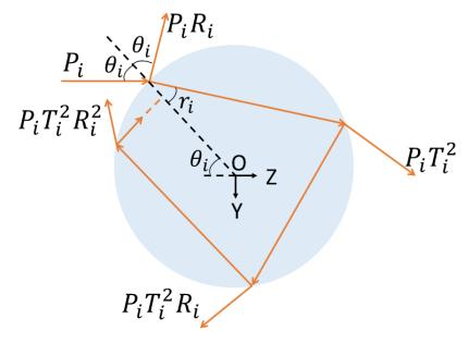
**Figure 2.** Calculation of the scattering and gradient forces acting on a Mie particle from a single ray, by taking into account geometrical optics and multiple reflection and transmission events, using Fresnel coefficients *R* and *T*.
