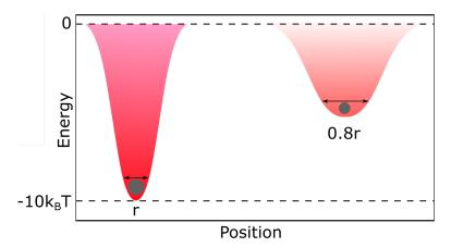
**Figure 4.** Graphical representation of the trapping potential wells for a polystyrene bead of radius *r* and 0.8*r*. A small decrease in the particle's size creates a significantly shallower and broader trapping potential well, which offers much weaker confinement and, thus, the particle has a higher probability to escape from the trap.
