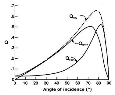
**Figure 3.** The calculated Q factors for the gradient, scattering, and total trapping efficiencies for a single circularly polarised ray acting on a spherical dielectric particle of effective refractive index  $n_{m,eff} = 1.2$ , as a function of the incident angle. Figure reproduced with permission from [28].
