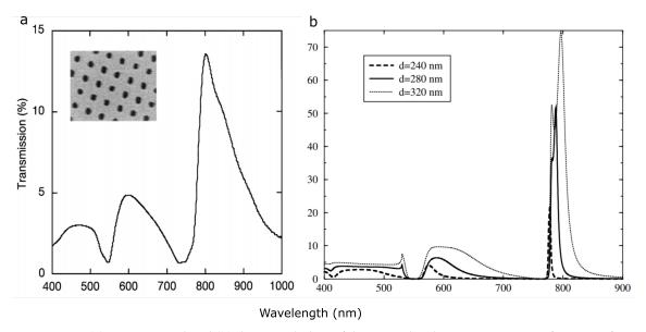
**Figure 8.** (a) Experimental and (b) theoretical plots of the normalised transmittance as a function of the incident light wavelength, for a square array of holes on a Ag thin film with thickness h = 320 nm. The diameter of the holes was d = 280 nm in the experiment and d = 240,280,320 nm for the calculations and the lattice constant 750 nm. Inset in the left plot shows an SEM image of the nano-hole lattice. Image reproduced with permission from [57].
