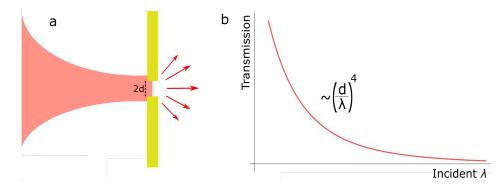
**Figure 7.** (a) Diffraction and transmission of visible light through a subwavelength circular hole of radius, d, on a perfectly conducting and infinitely thin metallic film. (b) According to Bethe's calculation the transmission of incident light  $\lambda$  scales as  $(d/\lambda)^4$ . Figure inspired by [59].
