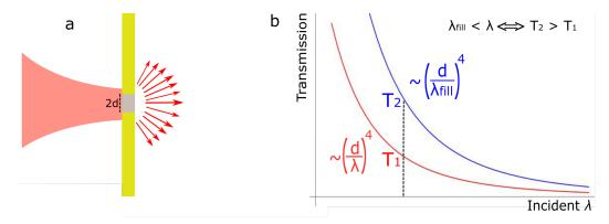
**Figure 9.** (a) The presence of a dielectric material of higher refractive index than the surroundings causes an increase in the transmission of light through the subwavelength aperture. (b) Shift of the transmission line due to existence of the dielectric material, leading to higher transmission  $T_2$ , compared to the transmission of light  $T_1$  in the case of non-filling. Figure inspired by [59].
