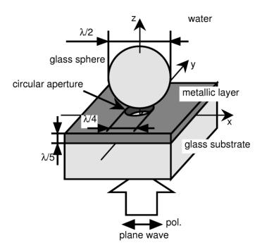
**Figure 5.** The geometrical model, studied by Okamoto et al., for subwavelength particle trapping, utilising the evanescent field near a metallic nano-aperture. This is the most commonly studied and reported geometry due to its simplicity to fabricate using the focussed ion beam (FIB) milling technique. Figure reproduced with permission from [38].
