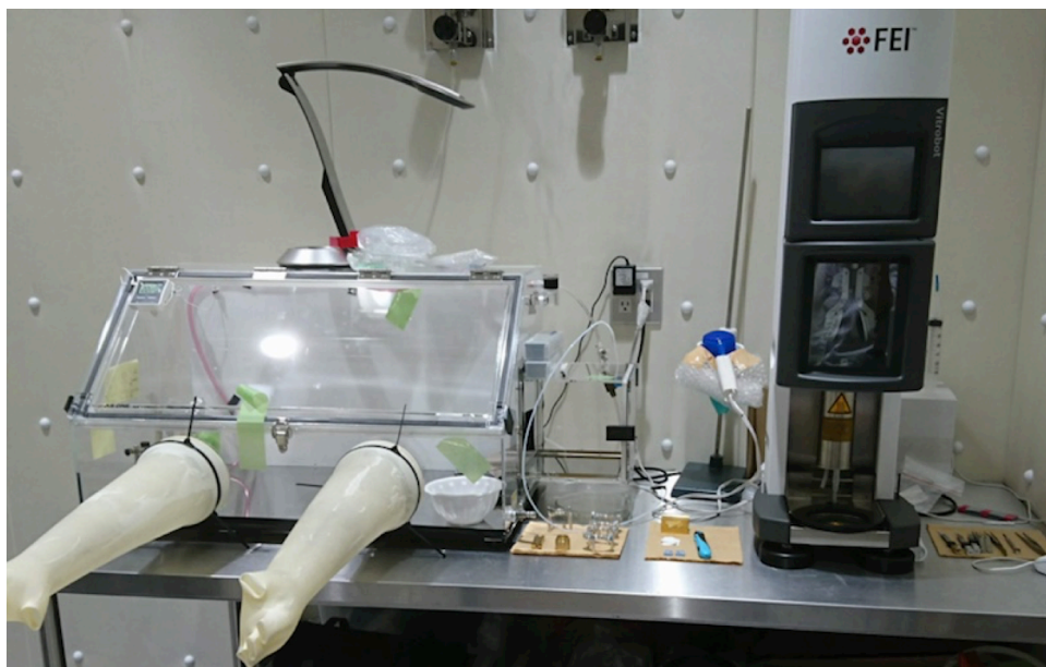
Figure S3. Cryo-sample preparation room situated at the Okinawa Institute of Science and Technology, Japan. All cryo-samples in this study were prepared in a dedicated preparation room to minimize moisture contamination. Before commencing sample preparation, the room was dehumidified to ~30% humidity. Sample grids were prepared by the plunge-freezing method in a semi-automated fashion with the FEI Mark IV Vitrobot (right) before immediate transfer to an N 2 -filled, positive-pressure glove box (left) located directly beside the Vitrobot. Humidity within the glove box was kept below 1% at all times. Transfer of the sample grid into the cryo-workstation and holder were conducted within the glove box, vastly reducing visible crystalline ice contamination, resulting in significant improvements in vitreous ice transparency (16).
