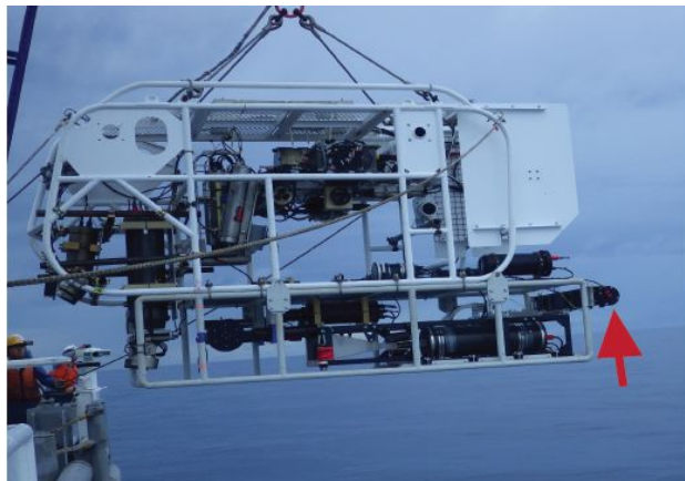
Figure 1.2. Photos of the JAMSTEC DEEP TOW 6KCTD (A) and BellaMare ISIIS small imager/area scanner attached to the DEEP TOW (B). Red arrows indicate the position of the ISIIS system on the DEEP TOW (A) and the imaging area of the ISIIS system (B). At each sampling station, the DEEP TOW was lowered straight down through the water column, to a maximum depth of 1000 m, before being towed at 1000 m and then continuing to be towed as it was raised back up through the water column. Only images from downward casts were used for this study, since forward motion of the frame prevented plankton from being properly imaged by the ISIIS.
