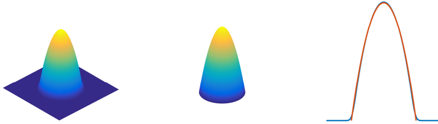
Figure 4.1: The numerical solution (left) and Thomas-Fermi (middle) solutions for a two-dimensional condensate of ^{87}\text{Rb} with N = 1 \times 10^5 atoms. The lineplot (right) is a central cut through both profiles showing the close match.
