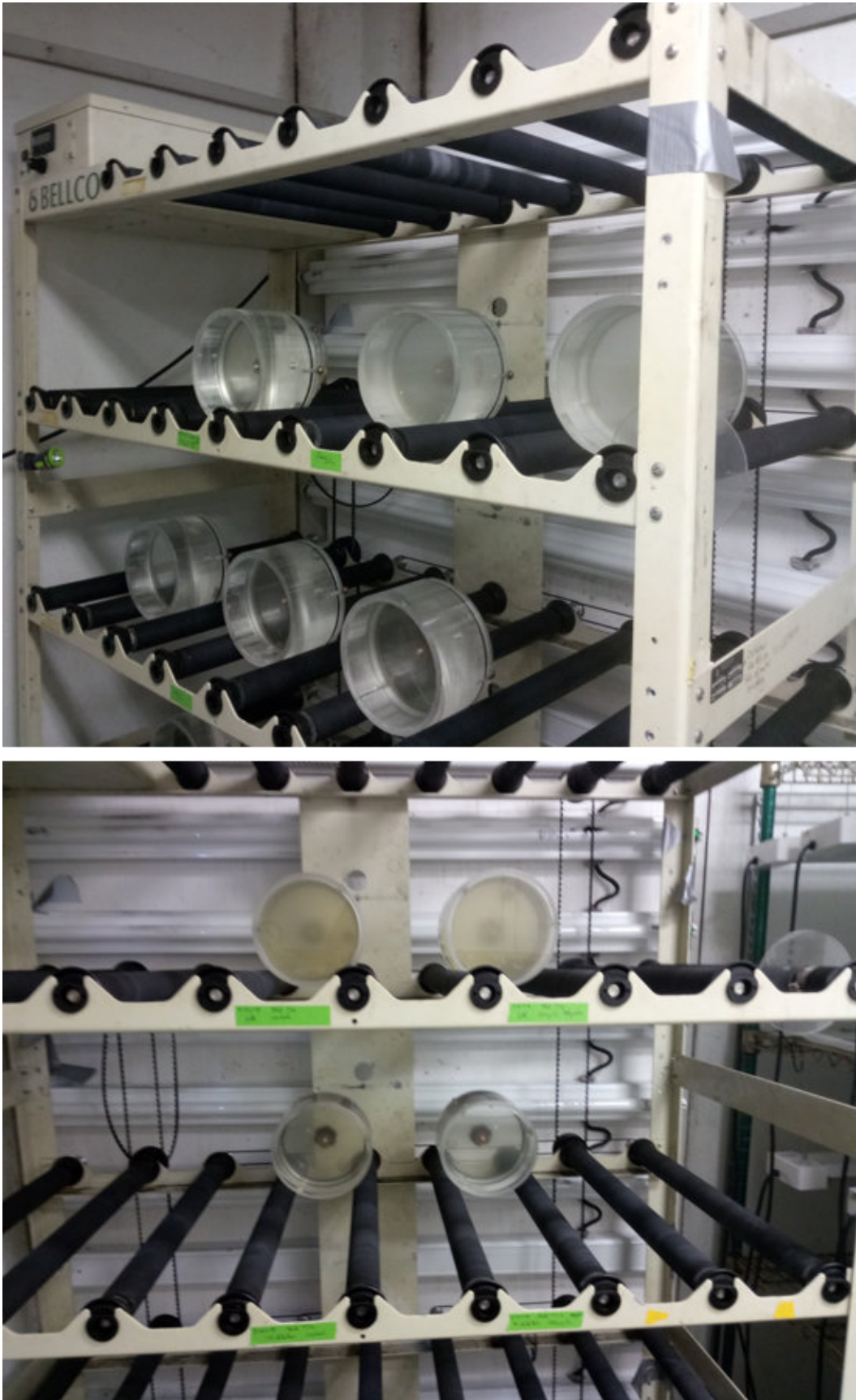
Figure 2.14: Rolling table for Skeletonema grethae in the climate chamber at 15°C in the dark.
