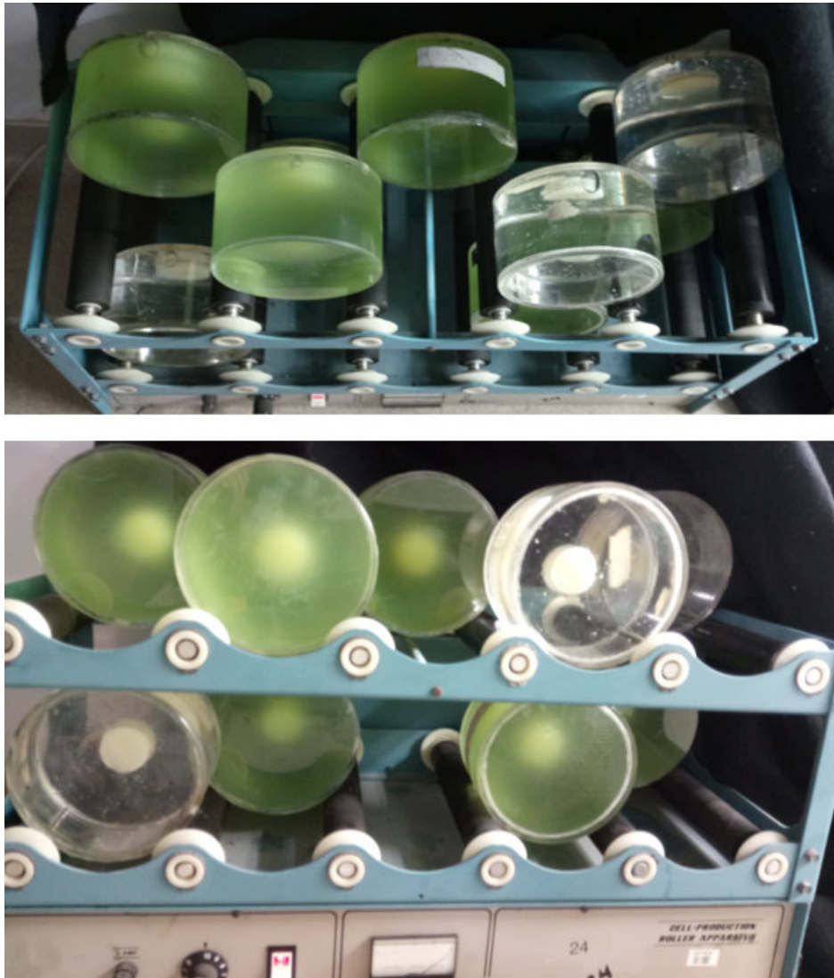
Figure 2.20: Rolling table setup for Synechococcus elongatus . To avoid artifacts in the data due to placement, one tank of each treatment was placed on the top and bottom levels.
