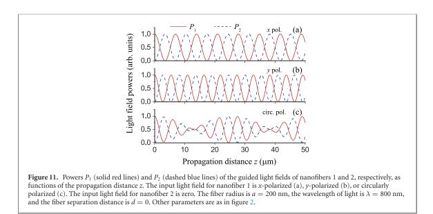
We note that transfer of power between light fields propagating in the guided modes of two parallel waveguides plays a very important role for the construction of practical optical devices, e.g. optical directional couplers, multicore fibers, wavelength-division multiplexers, polarization splitters, power-dependent nonlinear couplers, interferometers, ring resonators, and bistable devices [26–28].
