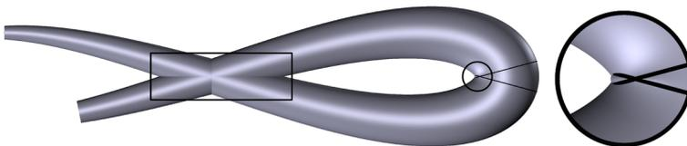
**Fig. 1** Local injectivity fails when adjacent material cross sections interpenetrate. This is illustrated in the *encircled region* (magnified on the *right*) where two material cross sections, traced on the surface, overlap, due to the excessive curvature of the midline. Global injectivity fails also when interpenetration occurs between cross sections that lie far apart along the midline. This situation, in which local injectivity is not hindered, is depicted in the framed region
