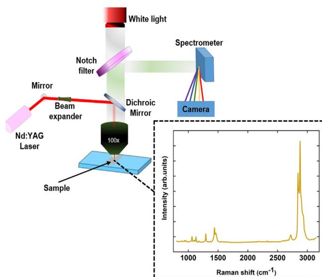
Fig. 2. A schematic illustration of the optical tweezers micro-Raman setup used in our experiments. Inset: characteristic spectrum of a polyethylene (PE) particle of 15  $\mu\text{m}$  diameter in a seawater environment.
