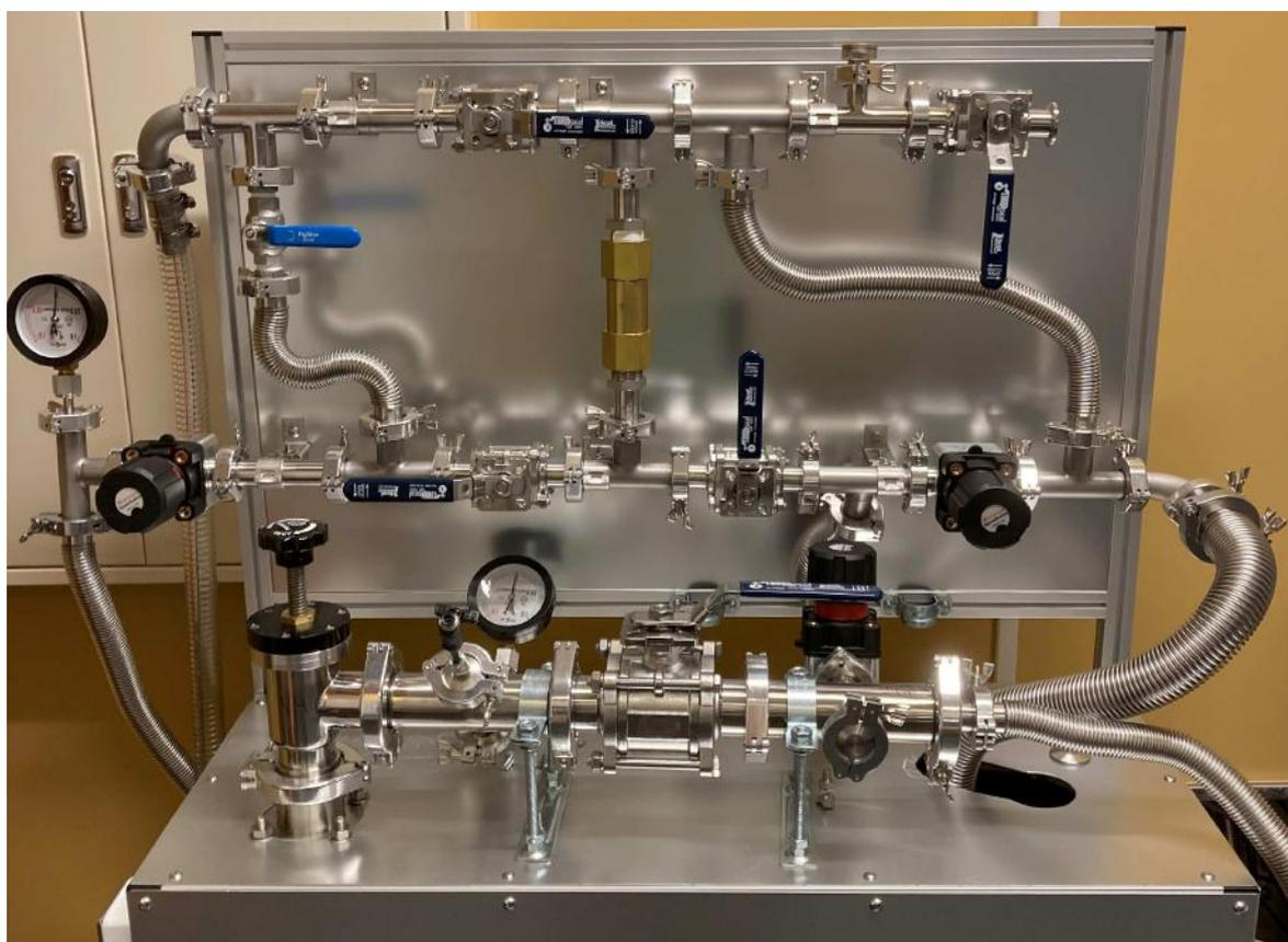
Photograph of one of the pumping stations in our lab. Note the pump and V13 are contained within the box at the bottom of the image.
