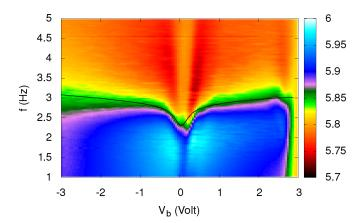
FIG. 3. Imaginary part of the cell admittance  ${\rm Im}\,Y/f_{\rm ac}$  (in arbitrary units) for the experimental parameters of Fig. 2; the admittance of the cell mainly behaves as a capacitance and is thus divided by  $f_{\rm ac}$  to compensate its linear increase with frequency. The position of the GMP resonance is given by the green contour curves, and the lowest eigenfrequency of the effective Schrödinger equation for  $\alpha=0.4^\circ$  is shown by the black line.
