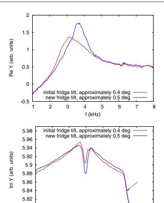
FIG. 8. The top panel shows that the frequency of the GMP mode can be changed by tilting the refrigerator, which modifies the angle  $\alpha$ ; the change in the resonance frequency is shown in the top panel with an increase in the resonance quality factor. The bottom panel confirms that the number of trapped electrons did not change as the refrigerator was tilted.
