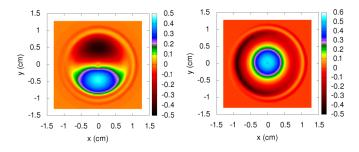
FIG. 5. Time-dependent part of the electron density as a function of the spatial coordinates x and y, calculated for the following parameters: saturation voltage  $V_{\rm sat}=0.8~{\rm V}, V_b=0~{\rm V}, V_d=7.5~{\rm V}, B=0.23~{\rm T},$  and  $f_{\rm ac}=2.5~{\rm kHz}$  (pentagon symbol in Fig. 2). The electron density has both an in-phase component  ${\rm Re}\,n_t$  (left panel) and an out-of-phase component  ${\rm Im}\,n_t$  (right panel) with respect to the excitation voltage.
