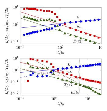
FIG. 2. Scaling laws for the bulk properties of the puff L (blue circle),  $u_L$  (red square), and  $T_L$  (green triangle, divided by a factor of 2 for graphical reasons), for (top) the shear-induced and (bottom) the buoyancy-induced fluctuation cases with  $\beta g T_0 L_0/u_0^2 \approx 0.05$  and 0.15, respectively. In the two panels, the solid and dash-dotted lines represent the expected scaling laws for the shear-induced and buoyancy-induced fluctuation regimes, respectively.
