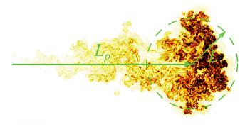
FIG. 1. Side view of a puff at  $t/t_0 \approx 5$  [corresponding to Re =  $L(t)u_L(t)/\nu \approx 4500$ ] from our simulation results. The color contour shows the magnitude of the vorticity field.
