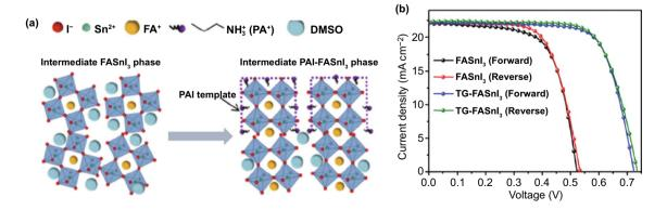
Fig. 7 a Possible mechanism of the template-growth process for FASnI<sub>3</sub> perovskite film. b *J-V* plots of the champion tin PSCs based on control and template-growth FASnI<sub>3</sub> perovskite absorbers. Reproduced with permission from Ref. [24] Copyright 2020 The Royal Society of Chemistry
