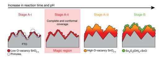
**Fig. 3** Schematic illustration of four major stages at different reaction time and pH value of the chemical bath deposition for SnO<sub>2</sub>, the magic region highlights the A-ii stage that exhibits an ideal film coverage, morphology and chemical composition of SnO<sub>2</sub> film. Reproduced with permission from Ref. [39] Copyright 2021 Nature Publishing Group
