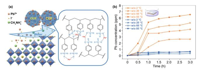
**Fig. 5** a Illustration of how CERs prevent the lead leakage via strong ionic interaction between Pb<sup>2+</sup> cations in broken perovskite films and the sulfonate groups. **b** Pb-soaking test results in water for the damaged perovskite solar modules without (yellow line) and with (blue line) the CER coating layer on glass side. Reproduced with permission from Ref. [50] Copyright 2020 Nature Publishing Group
