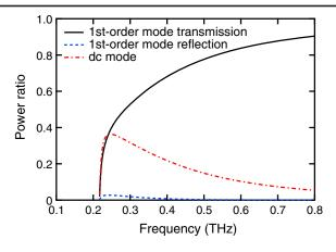
FIG. 2. Theoretically calculated first-order (l=1) power transmission (solid line), reflection (dashed line), and dc conversion ratios (dash-dotted line) as a function of the incident-wave frequency.
