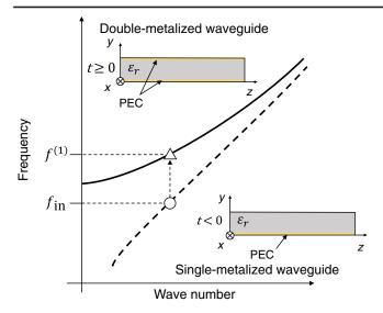
FIG. 1. Schematic diagram of dispersion relations between frequency and wave number in *z* direction for propagation modes in single-metalized (dashed line) and double-metalized (solid lines) waveguides. Insets show the geometric structures of single-metalized (lower one) and double-metalized (upper one) waveguides.
