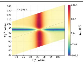
FIG. 2. Color map of the measured lateral displacement current  $I_{\text{later}}$  versus  $E_{\perp}^{(c)}$  and  $E_{\perp}^{(m)}$  for SEs under pulse-modulated  $(f_m = 200 \text{ kHz})$  excitation by 130-GHz radiation at T = 600 mK. The dashed line marks  $E_{\perp}^{(c)} = E_{\perp}^{(m)}$ .
