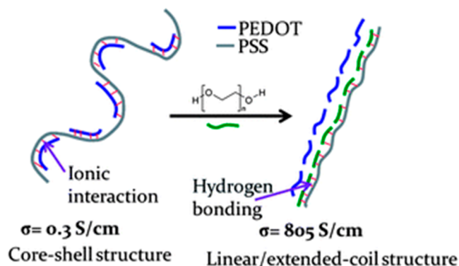
Figure 18. Schematic illustration of the molecular design strategy enhancement of conductivity incorporating PEG with PEDOT:PSS. Reproduced with permission from ref 196. Copyright 2013 Royal Society of Chemistry.
