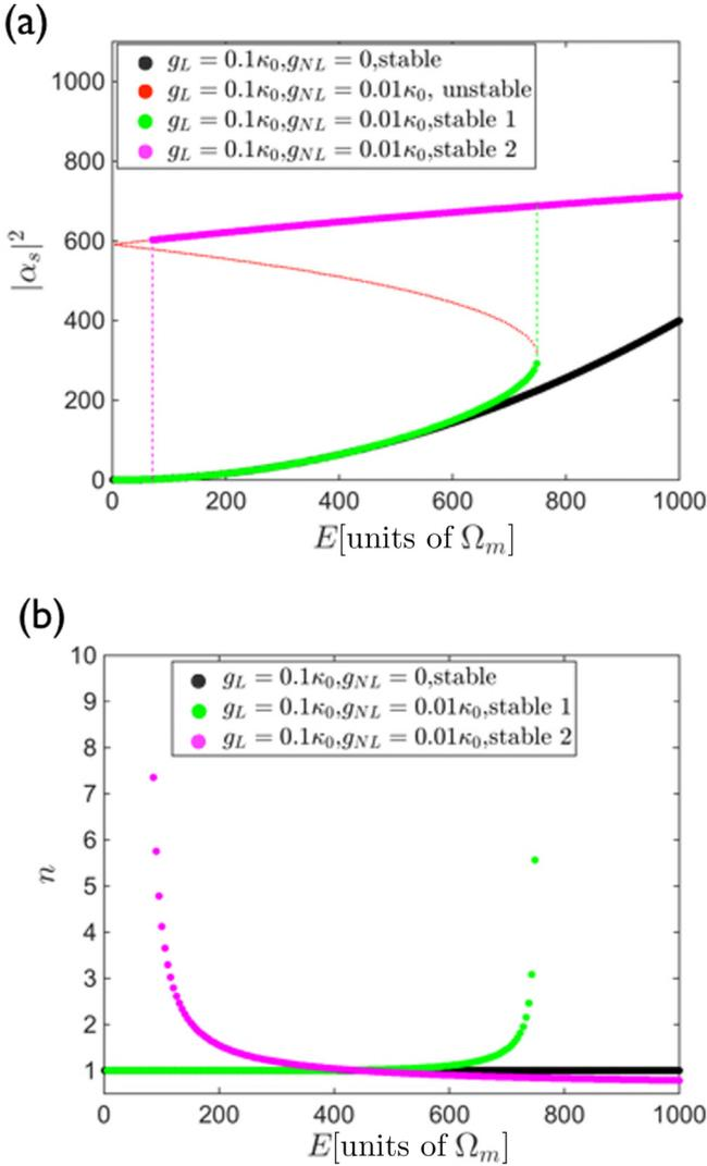
FIG. 3. (a) Photon number  $|\alpha_s|^2$  and (b) phonon number  $n$  as a function of  $E$  for both the linear and nonlinear case. The thin red (dotted) line corresponds to the unstable solutions, while the thicker lines are the various stable solutions.
