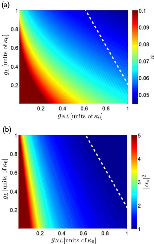
FIG. 5. (a) Phonon number  $n$  as a function of  $g_L$  and  $g_{NL}$ , where  $E$  has been chosen so as to minimize the temperature for each pair. (b) Photon number  $|\alpha_s|^2$  as a function of  $g_L$  and  $g_{NL}$  for the same steady-state solutions. The dashed white lines show where the photon number is equal to unity.
