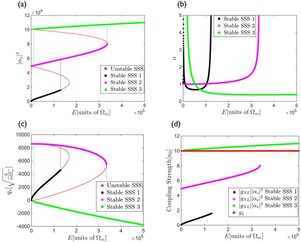
FIG. 4. (a) Photon number  $|\alpha_s|^2$ , (b) phonon number  $n$ , and (c) position of the membrane  $q_s$  as a function of  $E$ . The thin red line corresponds to the unstable solutions, while the thicker lines are the three stable solutions. (d)  $g_{NL}|\alpha_s|^2$  and  $g_L$  as a function of  $E$ .
