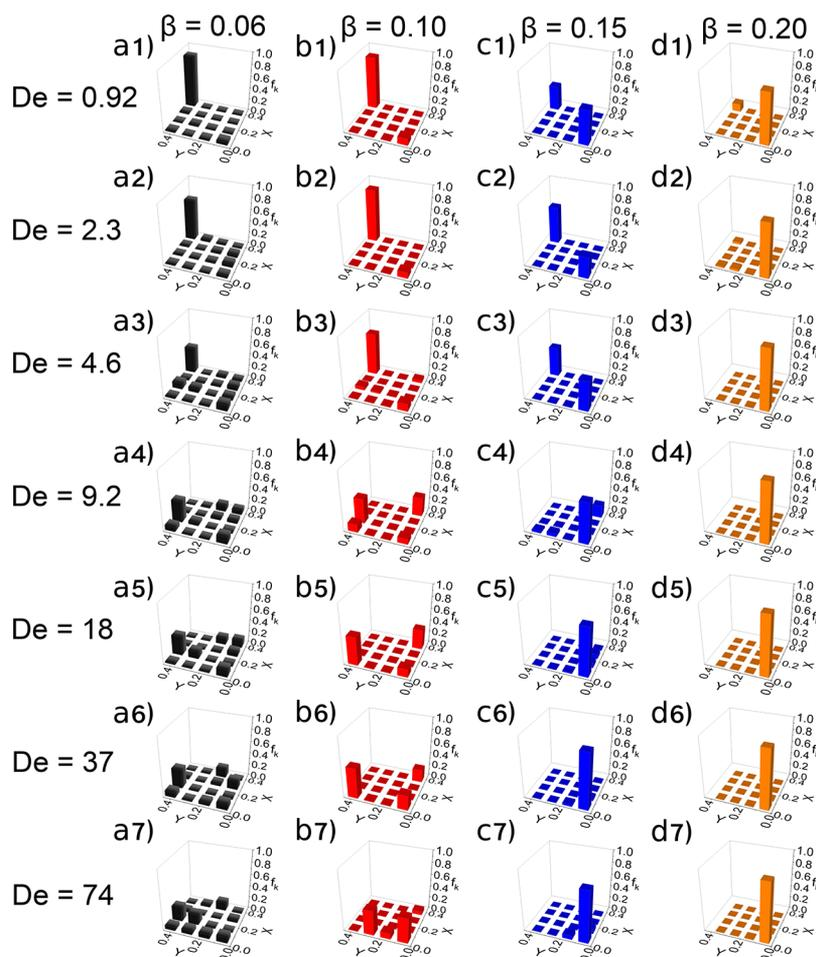
**Figure 5.** Migration of rigid particles strongly depends on the Deborah number and confinement ratio. Normalized fraction  $f_k$  of rigid particles at  $L_z = 7.5$  cm from the inlet as a function of the spatial coordinates  $XY$  in the upper-right quadrant of the channel cross section (see Figure 3d). Each row corresponds to a different Deborah number  $De$ . Each column corresponds to a different confinement ratio  $\beta$ .
