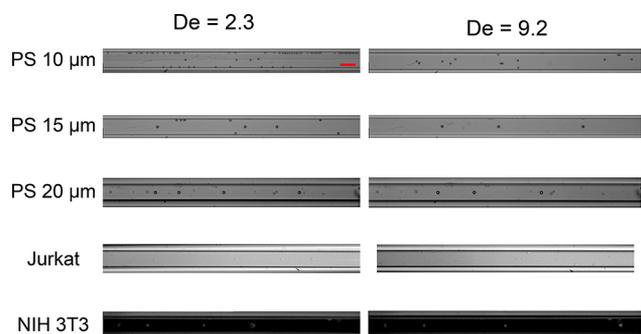
**Figure 4.** Experimental observation of particle and cell positions. Experimental images of particles and cells at  $L_z = 7.5$  cm from the inlet in the square-shaped microchannel. A  $10\times$  objective is used. Images of NIH 3T3 are obtained using phase contrast microscopy. Scale bar is  $100\ \mu\text{m}$ . Flow is from left to right.
