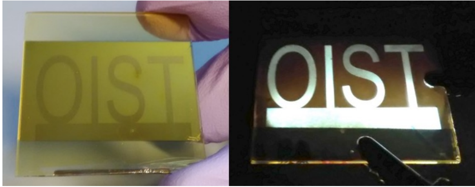
Figure S10. Large area CVD perovskite LED operated at 5 V.
